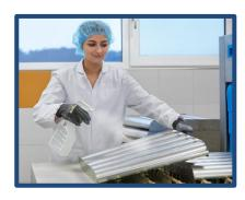
4 – Severely spoilt cassettes should be sprayed on both sides with a fat dissolving cleaning fluid.
