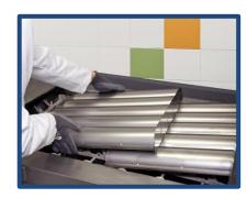
5 – Stand or lie the cassettes in the wash tray. Leave the cassettes to dry, any excess water can be removed with a dry cloth.
