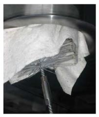
Place a cloth soaked in a foamy soap solution over the brush and clean the suction pipe. Intense soiling should subsequently only be cleaned with the brush. Then dry the damp suction pipe with a cleaning cloth over the head of the special brush.
