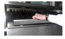
keep it horizontally to avoid any overflow. Dispose of the grease according to local regulations.
